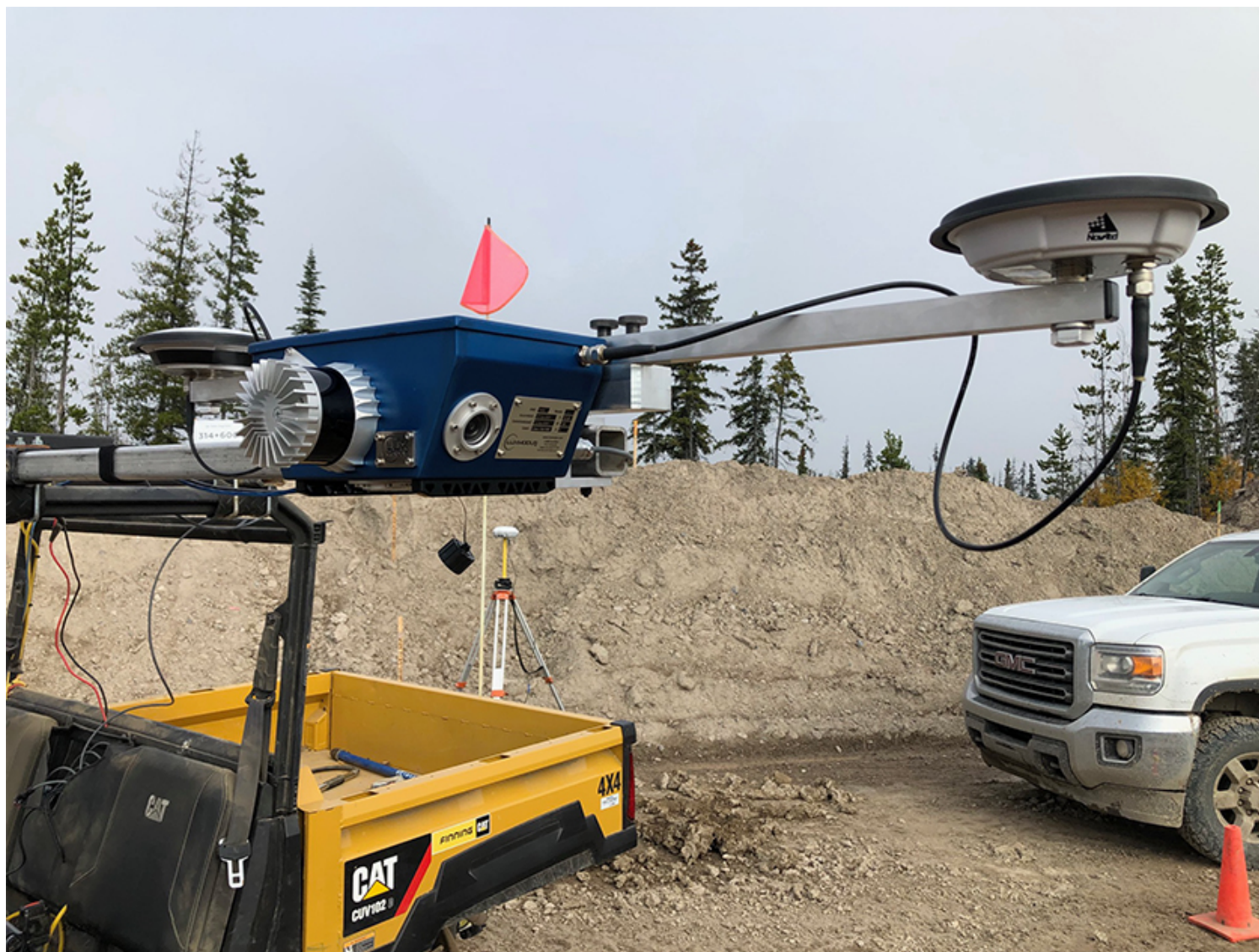
An Ouster OS1 sensor on a Lux Modus truck mount.
