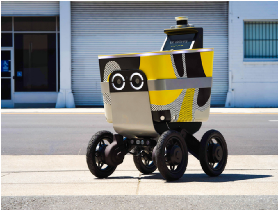
Serve Robotics next-generation robot outfitted with Ouster's OS1 digital lidar sensor (Photo: Business Wire)
