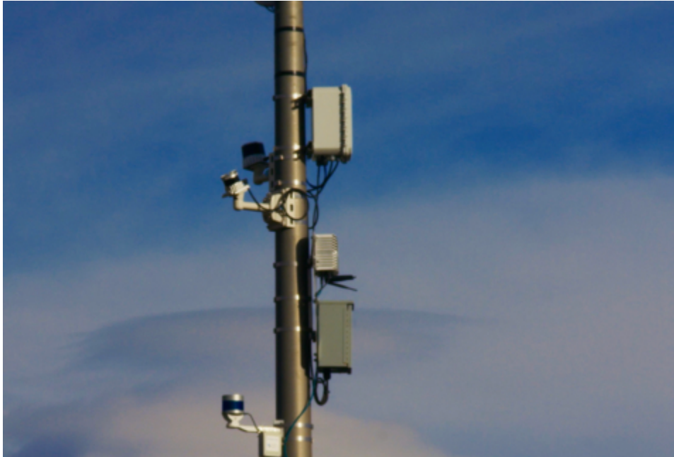
Ouster OS and Velodyne lidar sensors mounted at a traffic pole in Colorado. (Photo: Business Wire)
